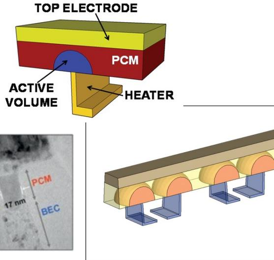
Ge-rich composition shifts  $T_x$  and data retention to higher temperatures (important for automotive applications)
